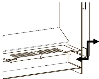
For best performance, it is important to empty the heater's ash pan after every use to keep the air opening under the grate open, allowing air to flow freely into the furnace.
