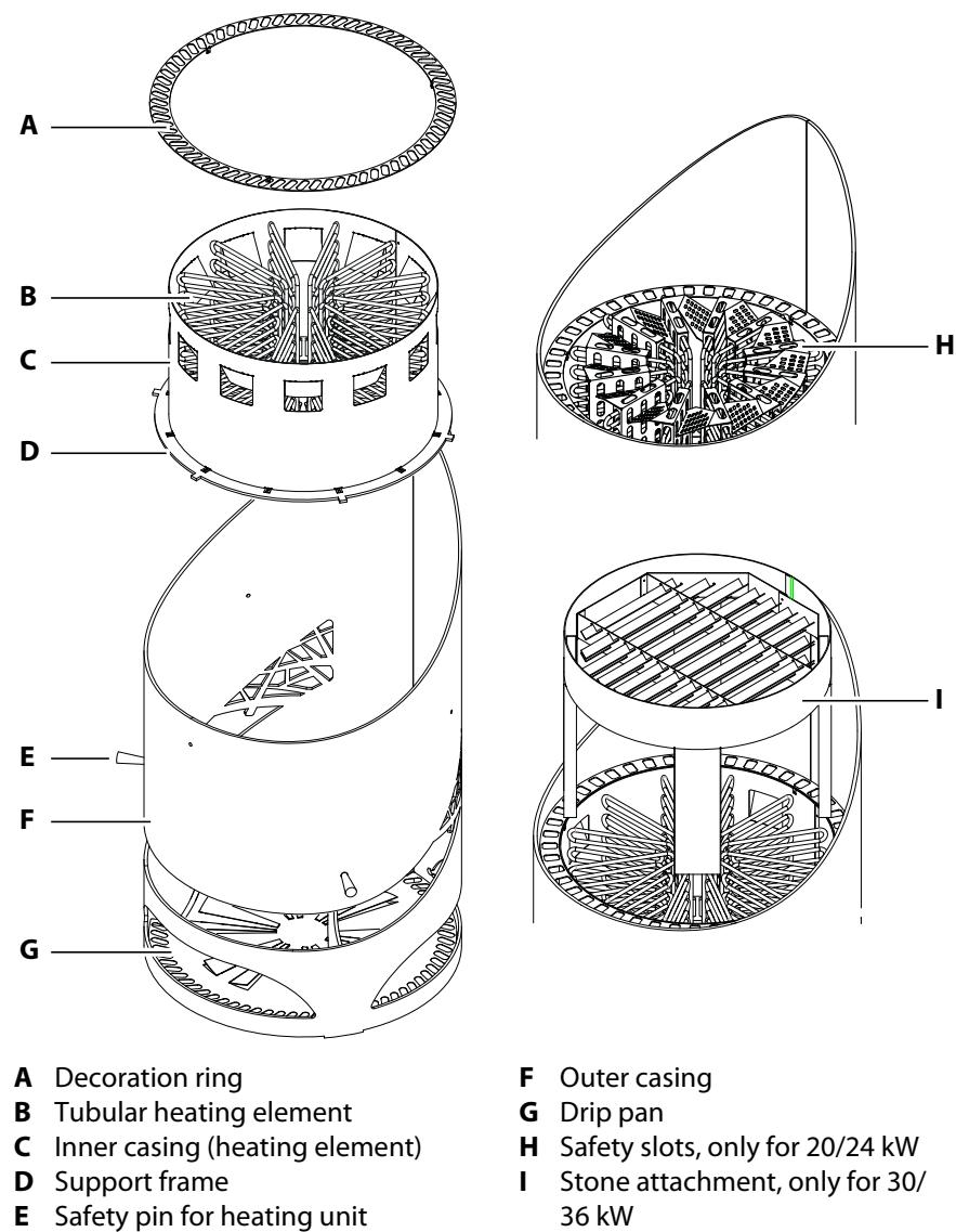
A drip pan is mounted under the heating element. It collects residual water from a water splash, which then vaporizes.
