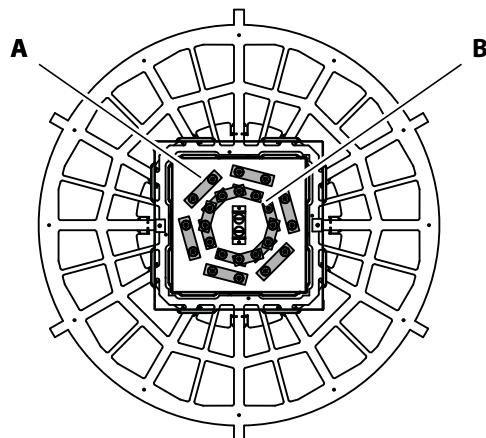
**A** Outer ring: 2 x 3 phases      **B** Inner ring: 2 x neutral conductors
