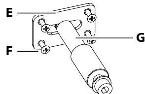
**E** Pre-mounted small plate      **F** Countersunk screw/crosshead screws
