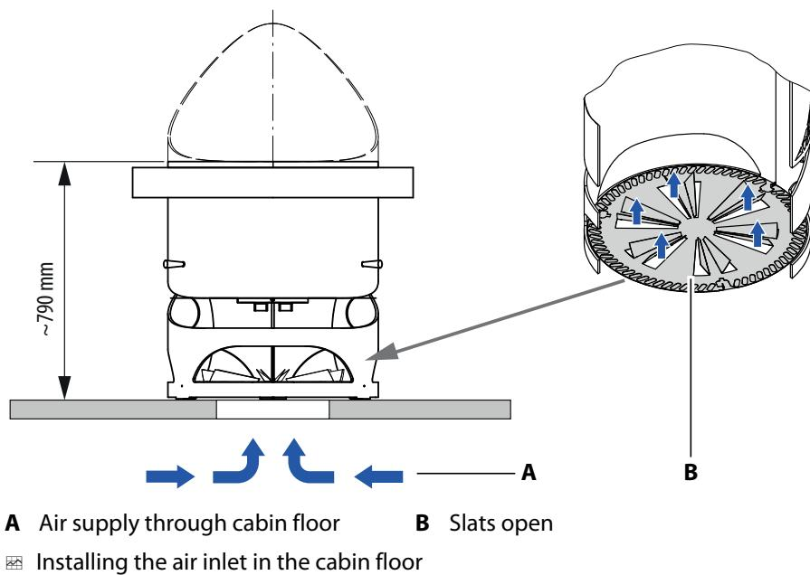
The slots are bent upward during heater manufacturing. They must be checked before commissioning.
