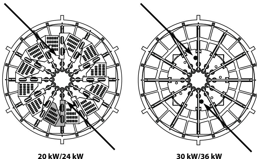
ⓘ To more easily reach the two screws on the 20 kW/24 kW model, the slots can be bent slightly to one side.
