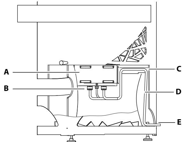
**A** Terminal box for the heating coil      **D** Connecting cable
