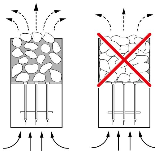
3 Place stones individually on the safety slots or in the stone attachment, ensuring there is plenty of space between the stones.
