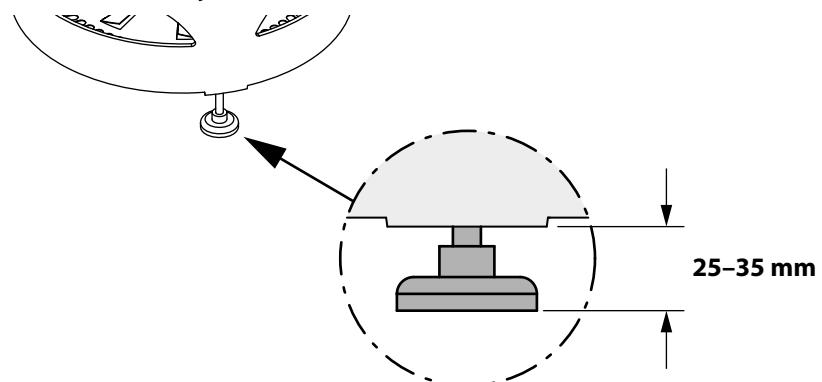
① Use a spirit level if needed to ensure that the heater is level.
