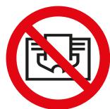
Objects placed on the heater can easily be ignited and cause fires.
